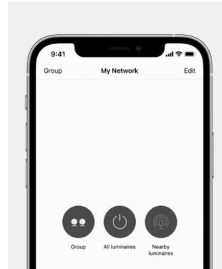
You can group luminaires together to make it easier to configure them. Within the group, you can define common settings, such as dimming and color temperature. There are two ways to create a group:
